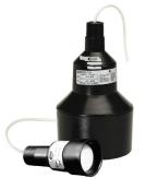
most versatile and powerful transducers in the industry. Our transducers have an accuracy of 0.25% of measured distance, or 1/4", whichever is greater, in approved applications. Available in frequencies of 22kHz and 43kHz to fit a variety of materials and distances. The range of Niagara sensors allows you to read levels from 1 to 2 feet to beyond 50 feet depending on sensor range. See table below. The transducer has a narrow beam angle, allowing it to be used in challenging applications.
