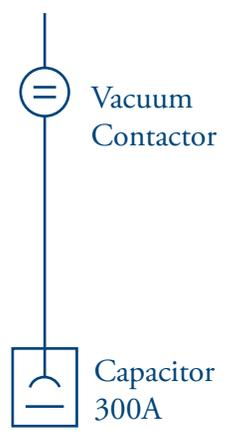
$$i \text{ max peak} = 1.41 \sqrt{I_{SC} \times I_1} = 1.41 \sqrt{20kA \times 300} = 3525 \text{ AMP}$$
