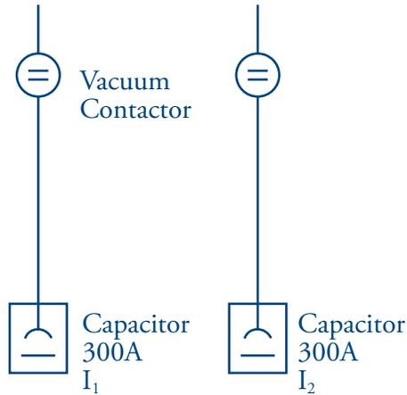
$$i_{\text{peak}} = 1235 \sqrt{\frac{(V_L) (I_1)}{L}} = 1235 \sqrt{\frac{0.6 \times 300}{10}} = 5236A$$
