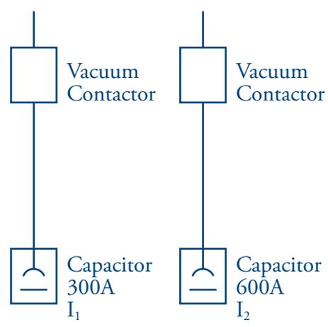
$$i \text{ max peak} = 1747 \sqrt{\frac{(V_L (I_1 \times I_2))}{L (I_1 + I_2)}} = 1747 \sqrt{\frac{.6 (300 \times 600)}{.1 (300 + 600)}} = 2,156,916A$$
