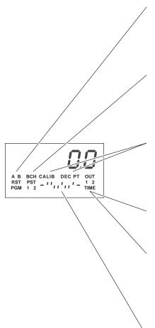
To start the Diagnostic display: turn power off, press and hold the Enter key, and re-apply power.
