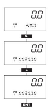
Use the Preset / Select key to display the Preset to be changed. Preset Data cannot be changed if Preset Data Lock, switch #4, is down.
