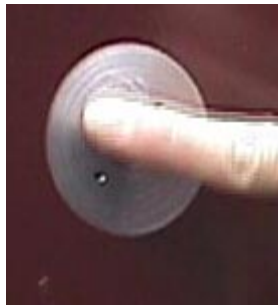
Fig. 3-10: Apply rust inhibitor.
