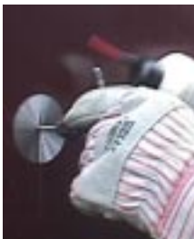
Figure 3-8: Thread the mounting hole using Tap and lubricating fluid.
