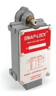
Double pole, double break, double throw, heavy duty limit switch having mechanical travel of 10° to trip and with two normally open and two normally closed circuit.
