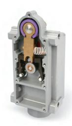
The contacts are positively maintained until the latch is disengaged by the return travel of the lever to reset the switch. The return spring serves to reset the switch automatically to its original position when the force on the operating lever is removed, but with the spring removed the operating lever will remain in either position as actuated.
