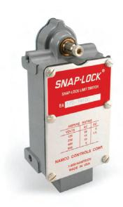
This heavy duty limit switch operates with two normally open and two normally closed circuits, with mechanical travel of less than 6½° required to trip.
