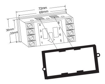
**Front Panel Installation** - Place the unit in the panel through the 33mm x 68mm cutout. Slide the included gasket over the rear of the unit, then slide the panel mount bracket into place so that the 4 tabs catch in the groves on the top and the bottom of the unit (the bracket should be oriented so that the tabs are on the side nearest the panel). Use the provided panel mount screws to tighten the bracket until there is a secure seal against the gasket.
