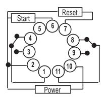
Warning: Do Not connect a coil in parallel with the start signal for the B506. Such a connection will cause the start signal to be continuously active. This situation also applies to the Reset input.
