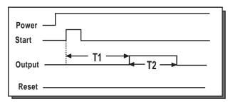
The delay cycle begins upon application of the start signal. The output will activate at the completion of the preset time (T1). Upon activation of the output the Interval cycle will begin. The output will be deactivated at the and the end of the Interval time (T2). T1 is the primary preset value and is set in Operation Mode. T2 is set in Program Mode in a range from 0.1 to 999.9 seconds. The timing sequence and output can also be reset through the reset input or interuption of power\*.
