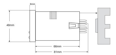
To wire the unit, an 11 pin socket is required. The unit can either be DIN rail mounted or panel mounted using the supplied mounting bracket. For panel mounting, place the unit in the cutout, then slide the bracket forward over the rear of the unit so that the tabs catch in the grooves on the housing and the bracket is as far forward as possible. Tighten the panel mount screws until there is a snug fit against the panel. Do not overtighten.
