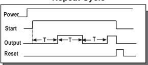
Timing begins on the leading edge of the start signal. A cycle is initiated where the output will be OFF for the preset time (T), then ON for the preset time. This cycle will continue until the start signal is removed, a reset signal is applied or power is interrupted\*. The unit can also be programmed for the timing sequence to begin with an ON cycle.
