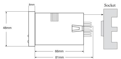
To wire the unit, an 8 pin socket is required. The unit can then either be DIN rail mounted or panel mounted using the supplied mounting bracket. For panel mounting, place the unit in the cutout, then slide the bracket forward over the rear of the unit so that the tabs catch in the grooves on the housing and the bracket is as far forward as possible. Tighten the panel mount screws until there is a snug fit against the panel. Do not overtighten.
