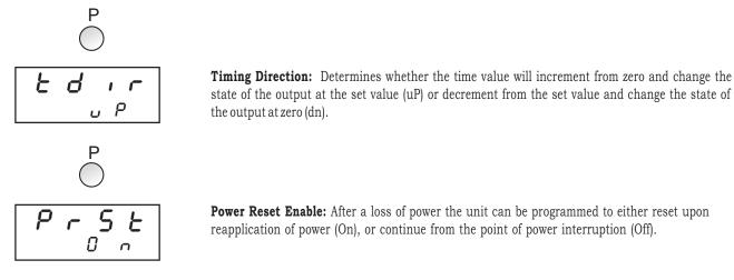
Power Reset Enable: After a loss of power the unit can be programmed to either reset upon reapplication of power (On), or continue from the point of power interruption (Off).
