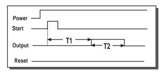
The delay cycle begins upon application of the start signal. The output will activate at the completion of the preset time (T1). Upon activation of the output, the Interval cycle will begin. The output will be deactivated at the end of the Interval time (T2). T1 is the primary preset value and is set in Operation Mode. T2 is set in Program Mode in a range from 0.1 to 999.9 seconds. The timing sequence and output can also be reset through the reset input or interruption of power.\*
