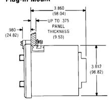
NOTE: PANELS THICKER THAN .140" REQUIRE ENLARGEMENT OF CORNERS TO ALLOW POSITIONING OF CORNER MOUNTING BRACKETS.
