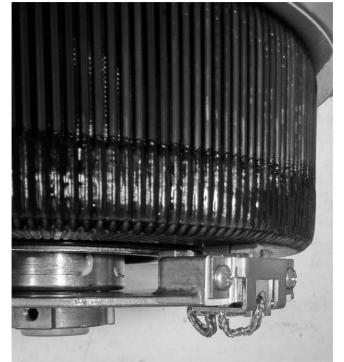
5. Remove the two (2) screws holding the brush assembly in place and discard the old brush assembly.
