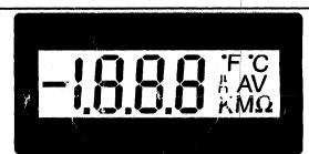
Features include 200mV full scale reading, programmable annunciators and decimal point, auto-polarity and operation from 5v or 9v supplies. In 5v mode each module generates its own -5v supply which enables it to measure signals with the same common zero as the supply. Connections are brought out to enable the module to operate in various modes including single ended, ratio measurement and differential. Different modes are selected by linking PCB solder pads which are provided for the purpose.
