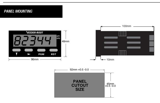
Mounting Grooves drawing above drawing drawing drawing above drawing dra
