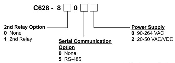
Additional outputs and options can be field installed through plug-in boards which can be ordered separately.
