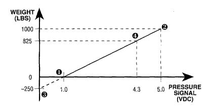
the Zero and Span adjustments for better accuracy.
