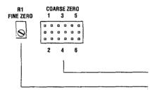
Jumper two pin pairs for coarse Zero display Adjust to set fine Zero display
