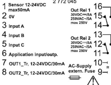
VDC 2 relays / 2 transistors
