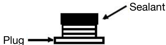
Figure 6. Preparing Supplied Plug for Unused Openings
