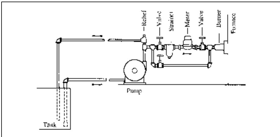
**C** – Installation on pump pressure oil burners having circulating system. Meter should be kept outside the circulating loop if possible. If two meters must be used on supply and return lines, first pump oil through the system with the burner shut off to check the exact uniformity of registration of the two meters. Be sure that the valve on the suction pipe is tight. The system must be air free to ensure the accuracy of the meters.
