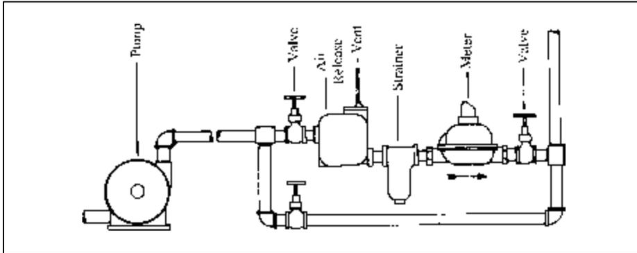
**B** – Pump pressure flow from the storage tank with pump, air release valve, strainer, meter, control valve, and riser pipe respectively. The air release may be omitted if the supply tank will never be emptied. If the supply tank is below the pump level, valves on the suction line must be tight. If the delivery tank is below meter level, a 1-foot riser pipe on the meter outlet should be used with a vacuum breaker or vent at the high point.
