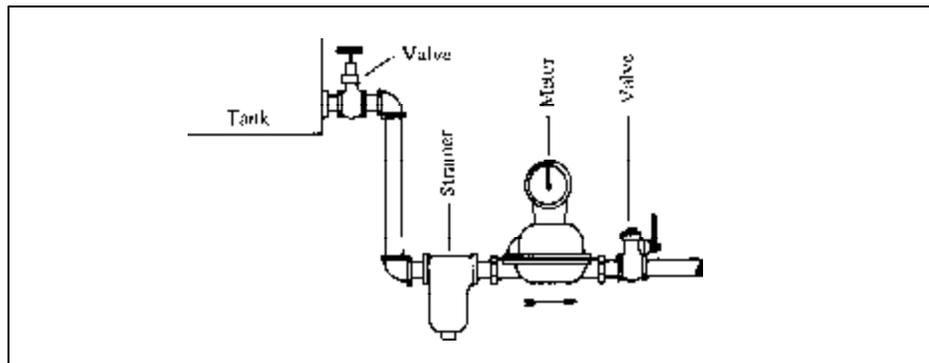
**A** – Gravity flow from storage tank with tank valve, strainer, meter, and control valve respectively. If there are many elbows or if very fast flow is wanted, the net drop should be at least two feet more.
